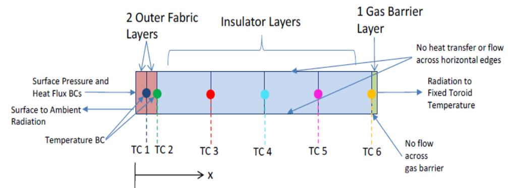
$$\rho_s C_{ps} \frac{\partial T}{\partial t} - \frac{\partial}{\partial x} \left( k \frac{\partial T}{\partial x} \right) + \rho_g C_{pg} v_{gx} \frac{\partial T}{\partial x} + H_d \frac{\partial \rho_s}{\partial t} = 0$$
