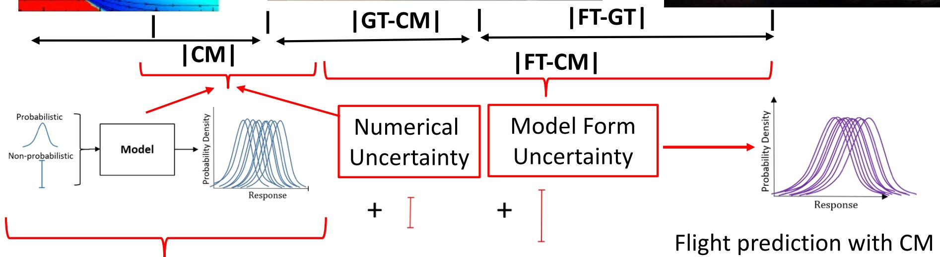
Model Input Uncertainty: Operating conditions, vehicle shape, parameters in turbulence models, chemical kinetics, ablation, radiation, etc.
